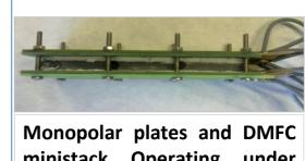
Monopolar plates and DMFC ministack Operating under passive mode for portable applications
